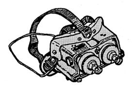
The goggles are a lightweight, battery-powered, passive night vision device worn on the head. It provides capabilities for reading, performing manual tasks, patrolling, and conducting surveillance. It has a built-in infrared light source used to provide added illumination for close-up viewing.
