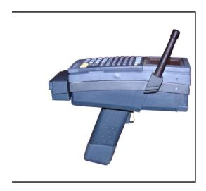
Figure C-11. Hand Held RFID Interrogator
