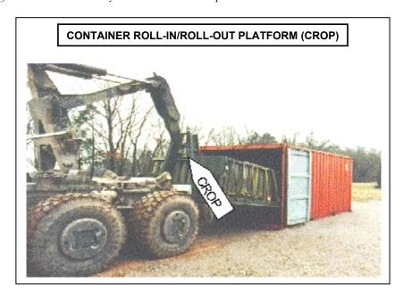
Figure J-17. Container Roll-In/Roll-Out Platform (CROP)
