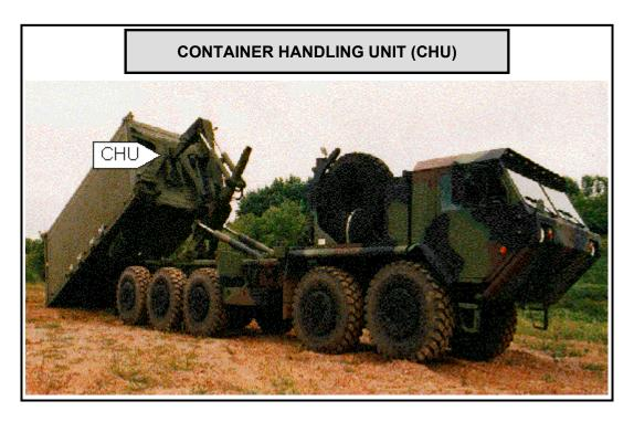
Figure J-7. Container Handling Unit (CHU)
