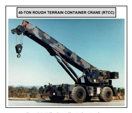
Figure J-3. 40-Ton Rough Terrain Container Crane
