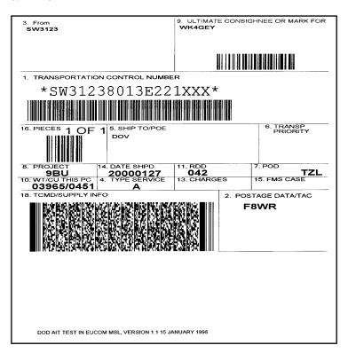
Figure C-3. MSL Using Both 2D and Linear Bar Code (example)
